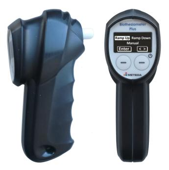
The Teflon (PTFE) or polyzene tactor on the rear of the device, which is the only part which comes into contact with the patient's skin, vibrates at a frequency of 100Hz for the length of the test, i.e. only few minutes.
